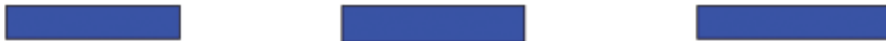
Figure 1 (Above): Markings for damage prevention purposes, in this case a water line.
