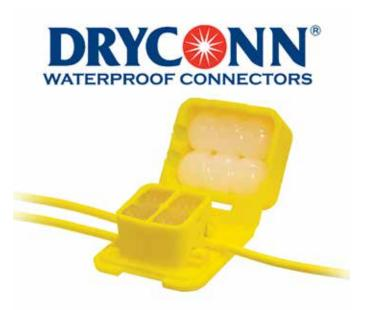
The DryConn® IDC makes waterproof tracer wire splices without the need for stripping wires! The connector's unique design allows for a service line to be installed without cutting the main line. Now the insulation displacement technology has made installation even easier by allowing connections to be made without stripping the conductor. Waterproof and corrosion proof, 50V, #14 – 12 Solid/Stranded Copper, Steel Core Tracer Wire, CCS.
