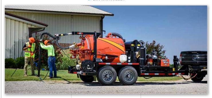
With its ease-of-use, high ROI and soft-excavation style, vacuum excavators are growing in popularity across a wide range of industries and applications. Today's contractors are using them to support HDD jobs, irrigation installation, and even landscaping and tree-care tasks. One reason for the growth is that present-day jobsites and underground environments are congested, with limited space and often many hazards. Vacuum excavators offer a solution to these problems.
