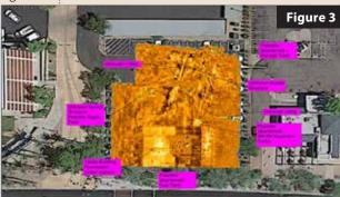
Figure 3, Multiple subsurface conflicts in addition to utilities discernable with MCGPR.
