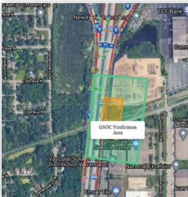
We can see the facility operator's centerline running through the right of way of a major highway, showing that this is an area that may require traffic control, or other support for locating. The facility operator data is displayed within the interactive map.
