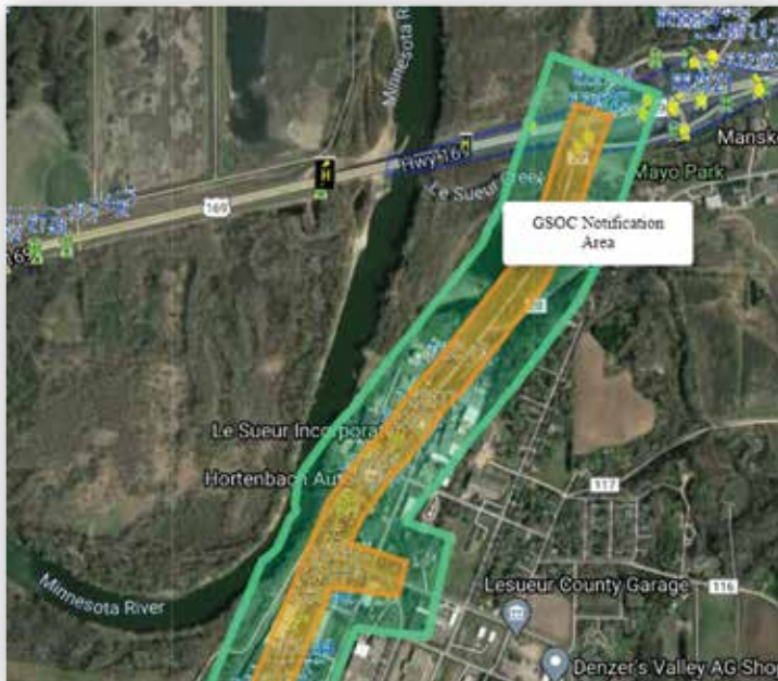
We can see the facility operator's centerline data intersecting the excavation area on the north end of the site.
