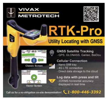
The vLoc3 RTK-Pro receiver is the first to add RTK GNSS accuracy to a utility locator. Using the RTK-Pro internal cellular module with 4G LTE capabilities, the operator can connect to the NTRIP RTK caster for RTCM 3 corrections. With these corrections, utility location data and the geographical location of the utility are collected with survey-grade accuracy.
